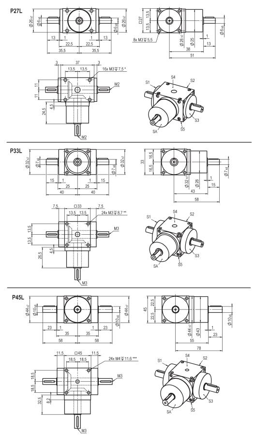
\*) thread starts from 4 mm depth, \*\*) thread starts from 4.5 mm depth, \*\*\*) thread starts from 6 mm depth, feather key to DIN 6885/1
