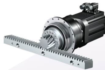
ZTRPH, ZTRPHV Rack and Pinion Drives with Servo Motors Module: 2 – 8 mm Feed force: 1.9 – 67 kN Feed velocity: 0.1 – 4 m/s High performance for demanding drive concepts.
